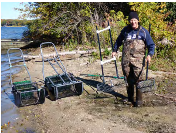
Figure 17. Small scale control devices maybe considered for removing zebra mussels in a clump form from swimming areas or sandy spawning sites.
