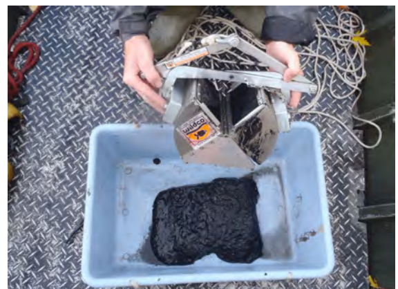
Figure A2b. Ponar dredge used to collect lake sediments in deeper water.
