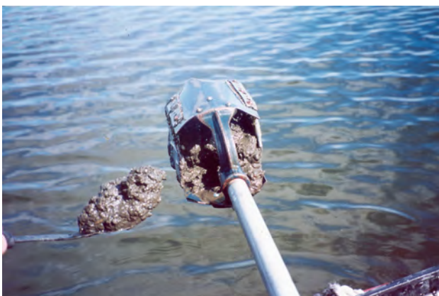
Figure A2a. Soil auger used to collect lake sediments in water depths to 10 feet.
