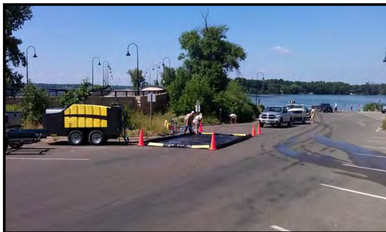
Portable boat decontamination unit and mat
