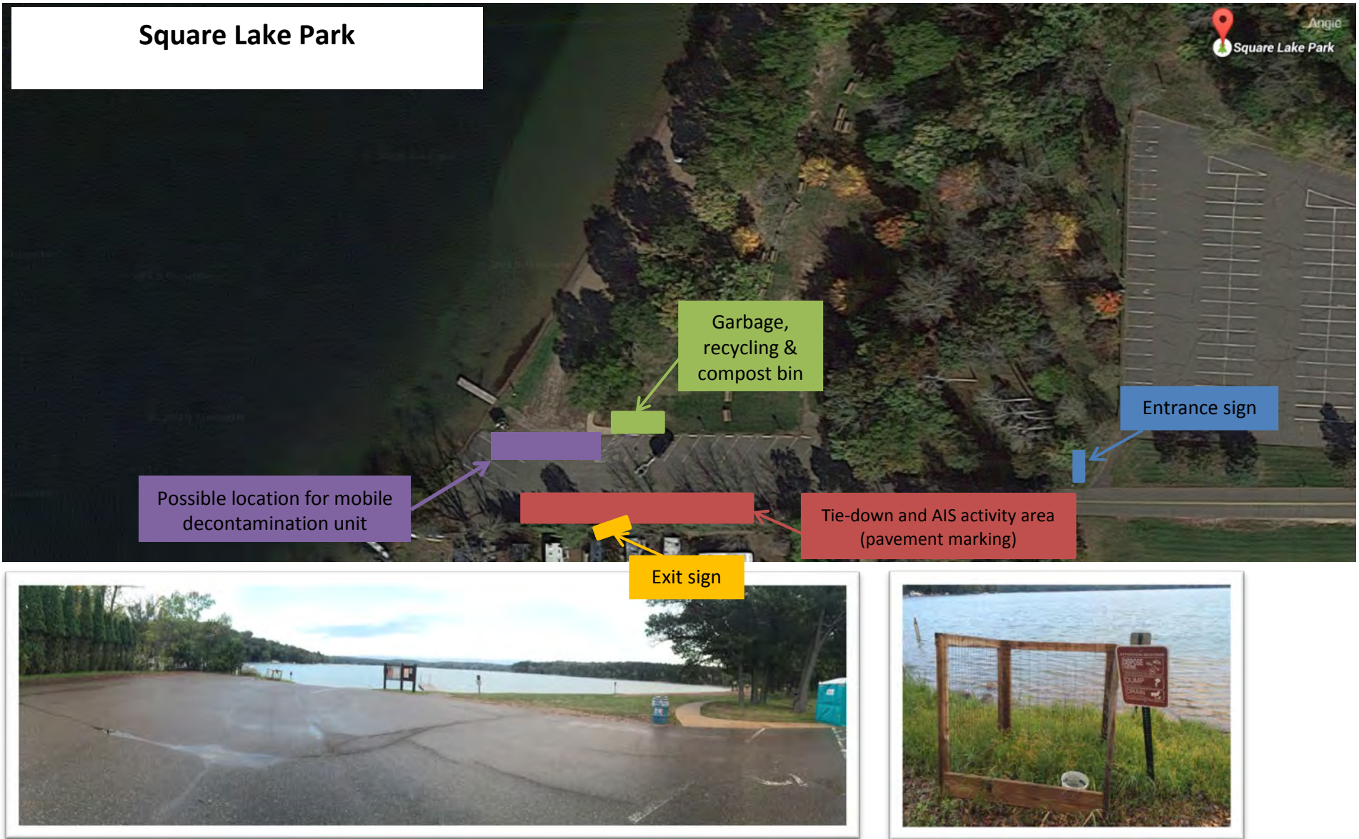
Above: New, free-standing, large entrance and exit signs have been added to prompt water users to clean and drain their boats before entering and after exiting the water. A mobile decontamination unit could be considered for high-use times. Existing compost bin will be relocated to increase use.
